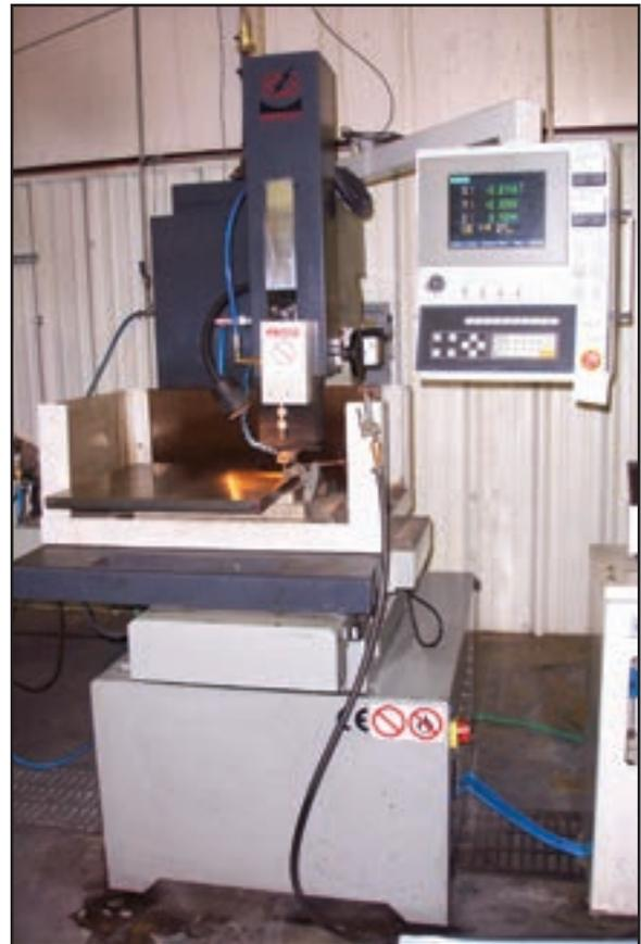
Small Hole EDM Drilling
