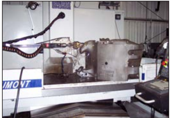
Beaumont Small Hole EDM: X—58.9 Inches, Y—30.5 Inches, Z—15.6 Inches Table Load 2,500 Pounds
