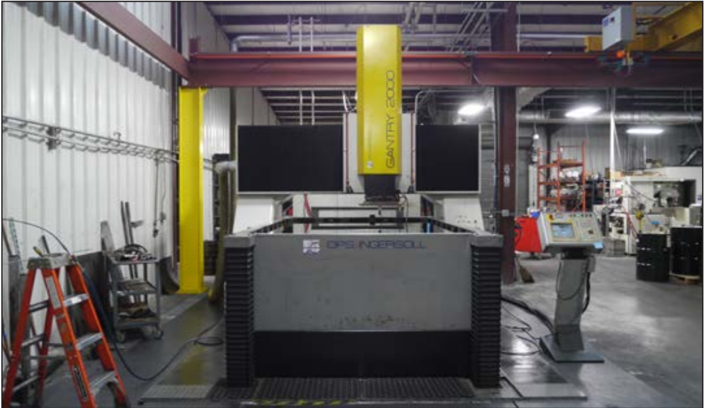
Ingersoll Gantry 2000 Work Tank: X—6.6 Feet, Y—10.6 Feet, Z—53 Inches (Area: Larger than a Ping Pong Table) Table Load 66,000 Pounds, Maximum Electrode 3,106 Pounds
