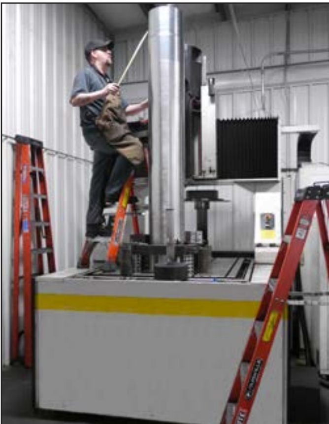
Ingersoll Gantry 2000 Work Tank: X—6.6 Feet, Y—10.6 Feet, Z—53 Inches (Area: Larger than a Ping Pong Table) Table Load 66,000 Pounds, Maximum Electrode 3,106 Pounds
