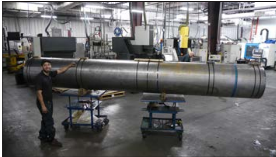
Split Large Tube Using Modified Wire EDM Diameter 27 Inches, Length 16.5 Feet
