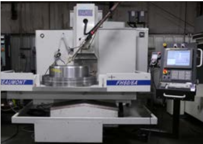
Beaumont Small Hole EDM: X—58.9 Inches, Y—30.5 Inches, Z—15.6 Inches Table Load 2,500 Pounds
