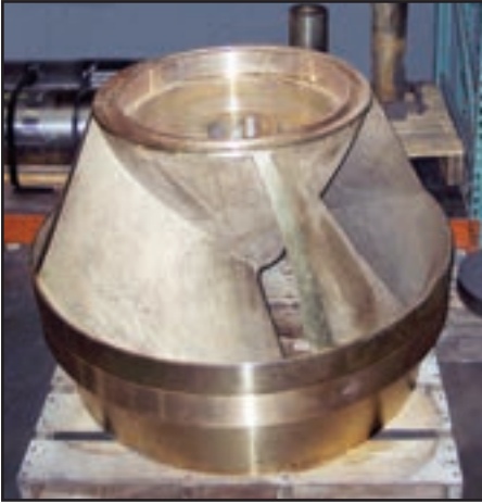
Keyway Large Bronze Turbine: Diameter 47 Inches, Height 34 Inches
