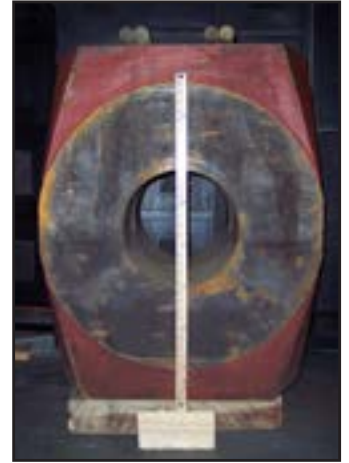
Test Specimens from Blowout Preventer 40 Inches Tall
